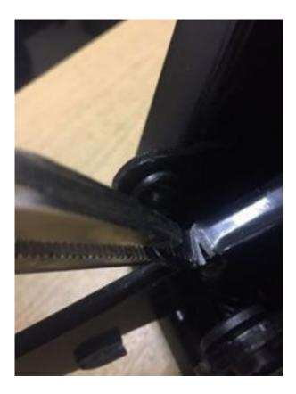
Once the bushes are installed, start by clipping the spring into the pedal bush.
