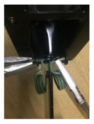
Once the spring is fitted into all 3 bushes, make sure it is seated centrally. If the pedal box 'tabs' are spread wide apart, they can be bent inwards to give a tighter fit as shown! (Pedal boxes are varying in dimension due to fabrication tolerances.
