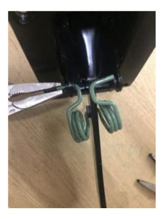
Now grip the other side of the spring and push it into the bush hole- on this side we prefer to pull the spring from the bottom of the footwell into place.
