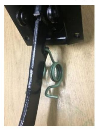
Rotate the spring round and use some good quality long nose mole grips or pliers to push the spring towards the bush.
